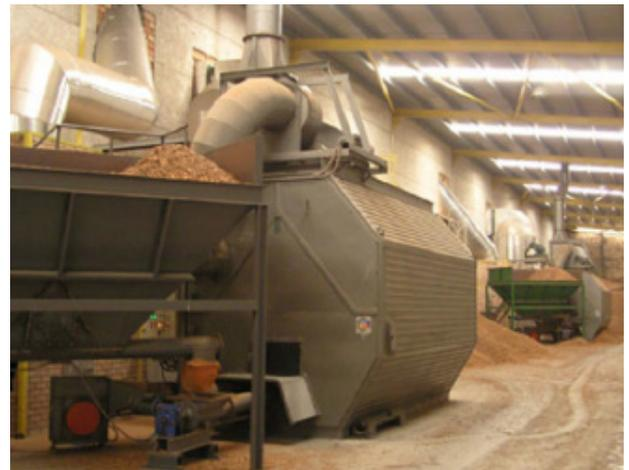
Figure 23: Biomass boiler at Briqueterie Samarra in Tangier (Beralmar, 2015)
